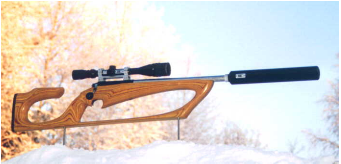
Photo of a custom built BR Integral rifle with a Telescopic Reflex Suppressor.
