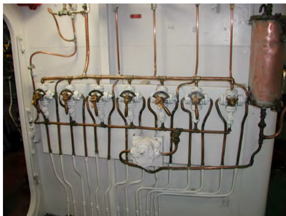
Cross Flooding Controls
