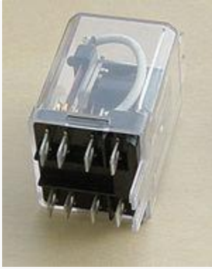
A DPDT AC coil relay with "ice cube" packaging
