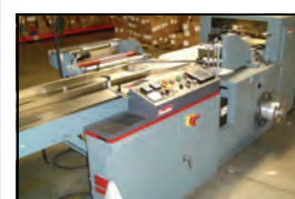
Shanklin HS-1 Wrapper Side Seal / Year 2002 w/T-71 Tunnel 8' Lugged Infeed Speed: 100 pkg/min
