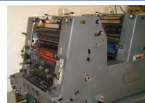
Heidelberg GTOZ52 1985 2-Color Offset Press Kompac Dampening Includes: Plate Punch Numbering Attachments
