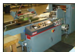
Shanklin F-5A Wrapper Side Seal / Year 2002 SLC-503 Controller 12' Lugged Infeed Speed: 75 pkg/min
