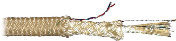
Fig 3-5. A Braided Rope with Hollow Braided Core
