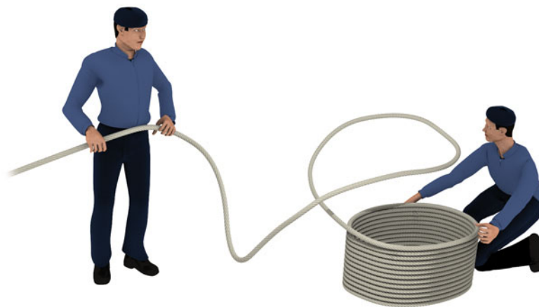
Fig 3-28. Running Out a Coiled Down Wire
