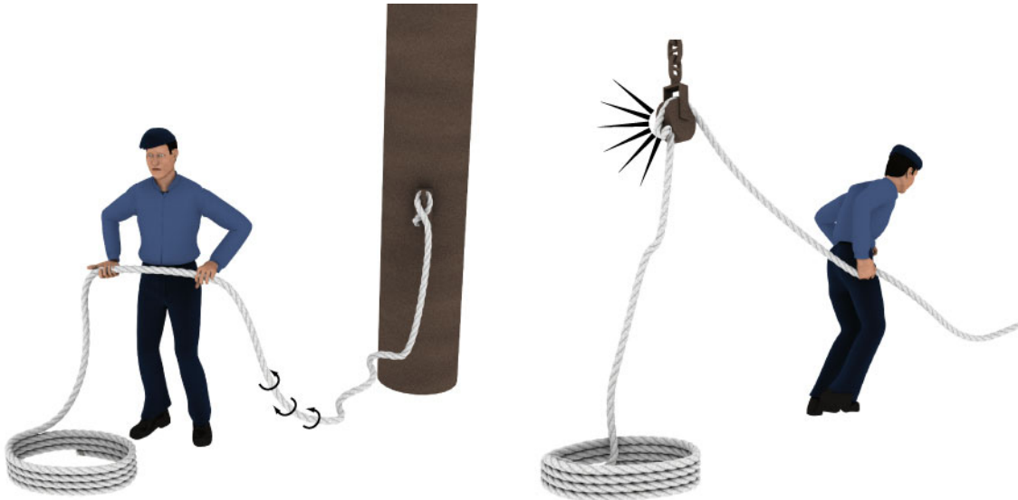
Fig 3-13. Mistakes in Coiling Down
