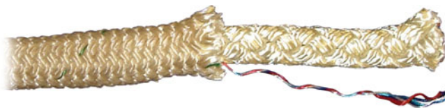
Fig 3-6. A Braided Rope with a Multiplicity of Three Strand Rope Core Members
