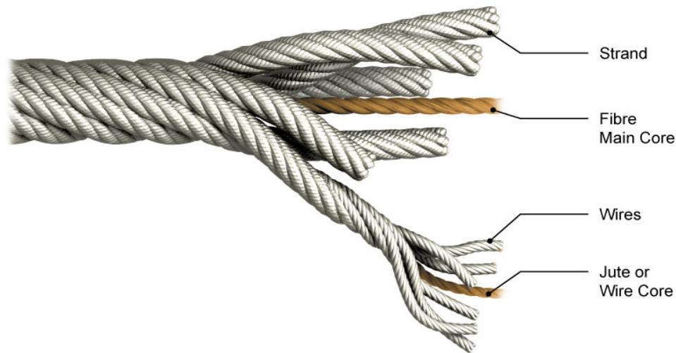
Fig 3-7. Construction of a Wire Rope
