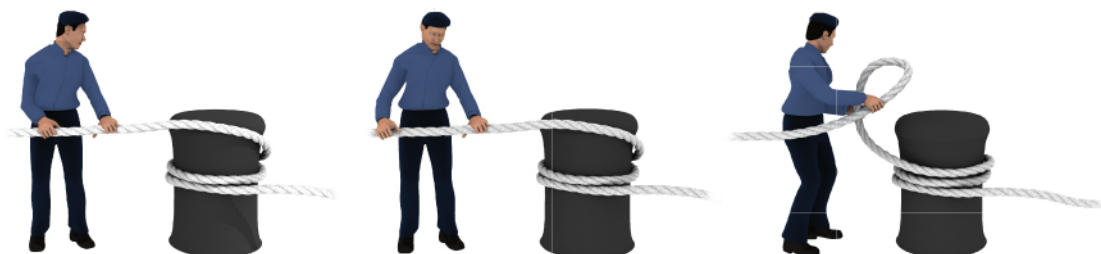
Fig 3-44. Catching a Turn on a Single Bollard
