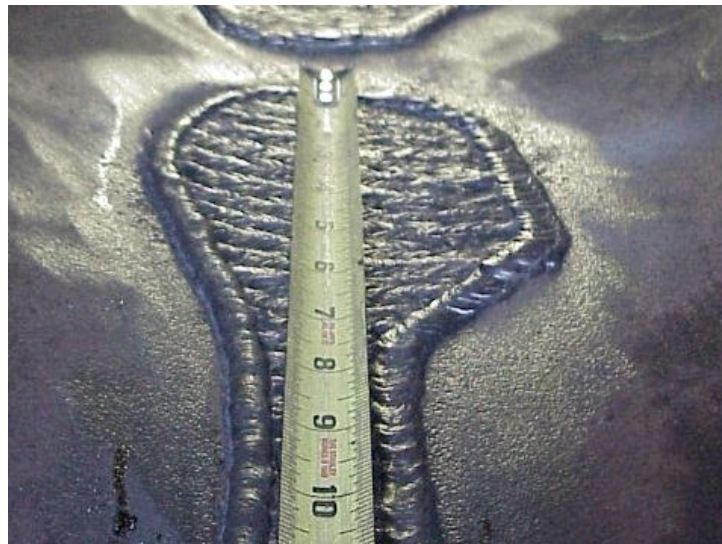
Figure 5. Appearance of typical completed weld deposition repair
