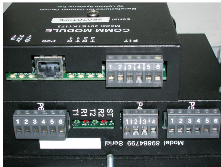
Figure 12 – Analog Input (P17) and Ethernet (P20) Connectors
