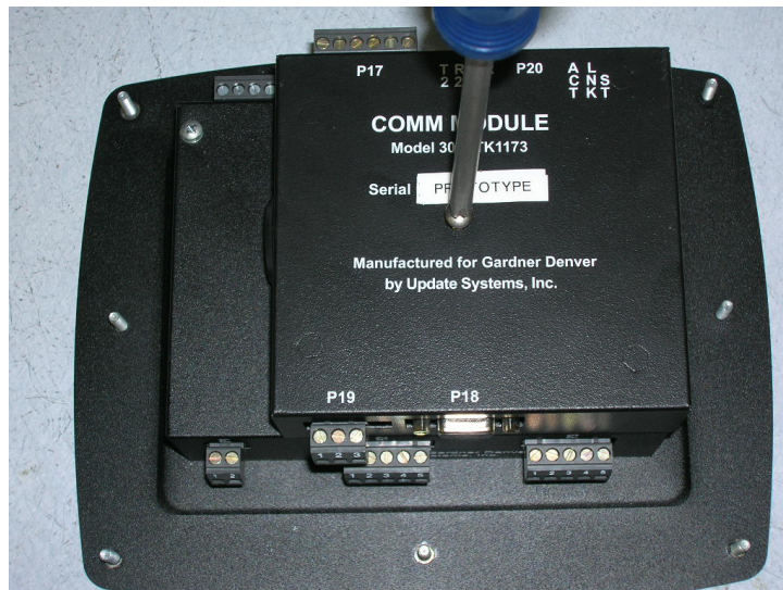
Figure 4 - Tighten Captive Screw
