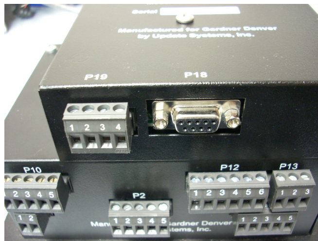
Figure 8– Serial (P18) and Network (P19) Connectors
