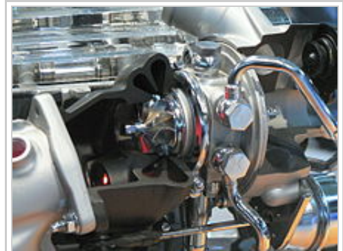
Cutaway showing a radial-inflow turbine that looks similar to the turbine shown in Figure 3.1
