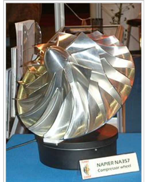
Centrifugal impeller with a highly polished surface likely to improve performance
