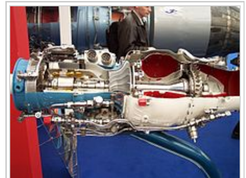
Jet engine cutaway showing the centrifugal compressor and other parts
