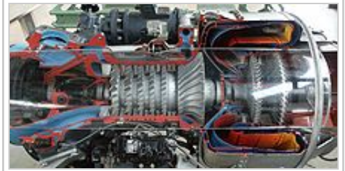
Cutaway showing an axi-centrifugal compressor gas turbine
