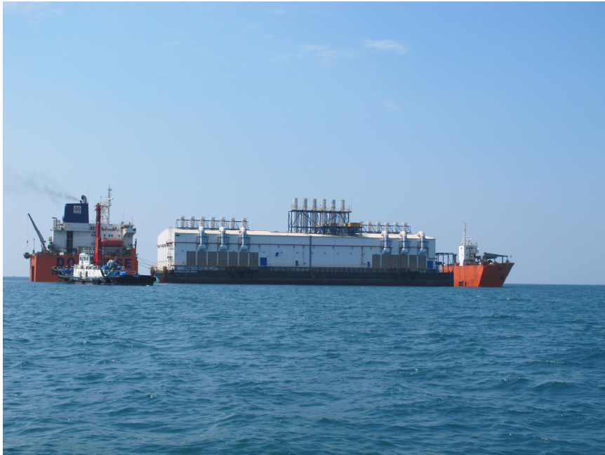
Barge loaded on submersible vessel - November 30, 2011 During transport, all internal equipment and components were fastened.
