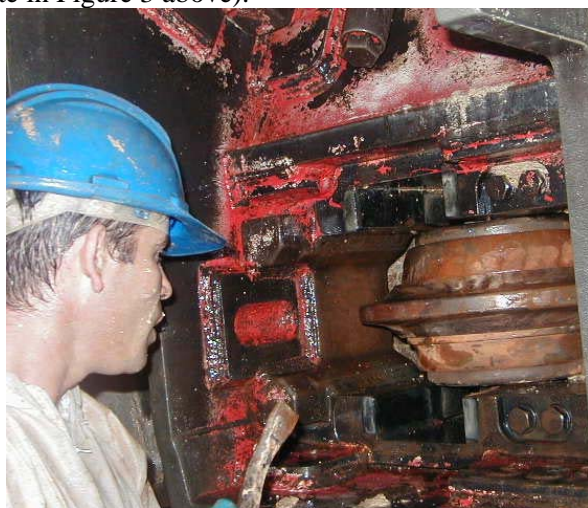
The consequences of this approach were the rapid wearing of the cutting tools and the structure of the cutterhead. By the time the TBM had reached the 24 do Agosto station, much of the front and periphery of the cutterhead had to be rebuilt underground, stopping progress on the tunnel drive for an additional 6 weeks (note in Figure 3 above).
