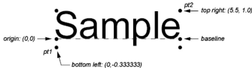
The next figure shows the point values that `acedTextBox()` returns for samples of vertical and aligned text. In both samples, the height of the letters was entered as 1.0. (For the rotated text, this height is scaled to fit the alignment points.)
