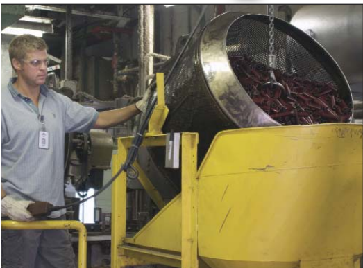
Mechanical adjuster Tim Ryman moves waxed tubes into the curing room.
