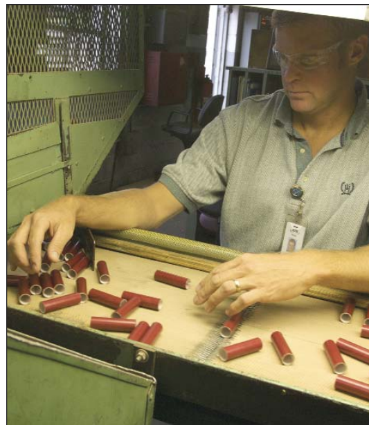
The cut tubes are being inspected manually by Tim Ryman. Any with flaws are weeded out.
