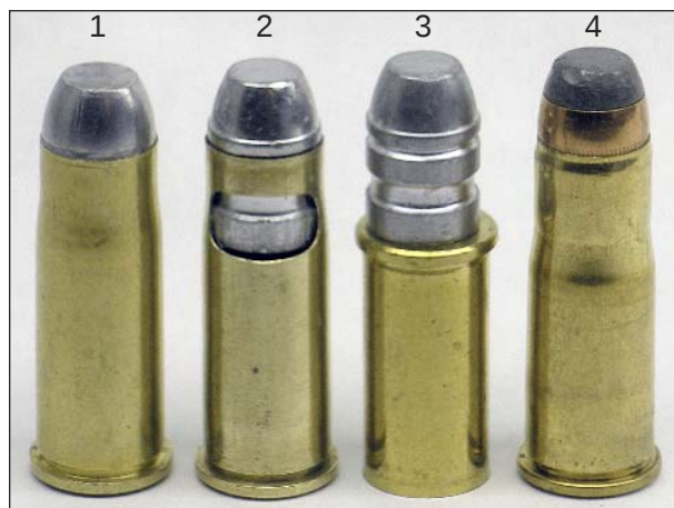
A .38 WCF handload (1) with a short case neck is shown with the RCBS 40-185-SWC (3) in a partially sectioned case neck (2) to show how the lubrication groove and base band extend below the case neck. A factory load (4) is shown for comparison.
