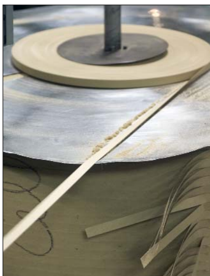
The basic material for the traditional paper base wad comes in a large spool, like tape, and is tightly wound into a base wad.
