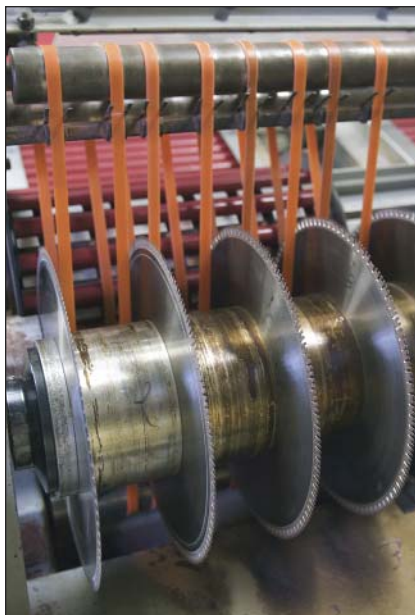
The 11-inch tubes go into the cutting machine and emerge as 2¼-inch tubes.
