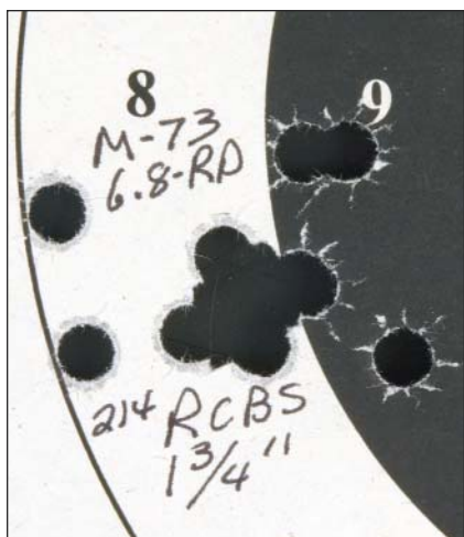
Left, Mike considers RN/FP bullets to be as inherently accurate as any other design, all other factors being equal. This 50-yard group was fired with a Cimarron Model 1873 .44 WCF rifle. Right, a Colt SAA .44 WCF fired this group at 25 yards from a machine rest.
