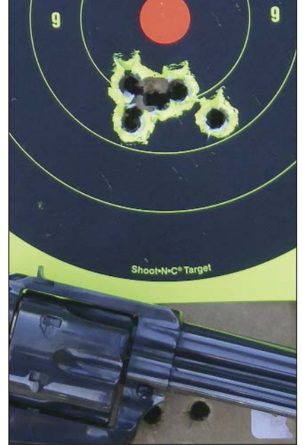
Above left, this Savage Model 10 .223 Remington stoked with Nosler 55-grain Ballistic Tips and 24.5 grains of AA-2230 powder offers fine accuracy potential. Right, a custom Colt-pattern SAA Flattop Target .44 Special produced this 25-yard group using 9.3 grains of AA-5 with the 250-grain Lyman/Keith cast bullet 42921.
