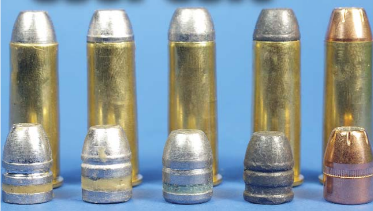
These bullets were shot in the Colt Lightning. From the left: Lyman 42798, RCBS 44-200-FN, Laser-Cast 200 RN FP BB .427 inch, CMC 200 RNFP .429 inch and Hornady 200-grain XTP.
