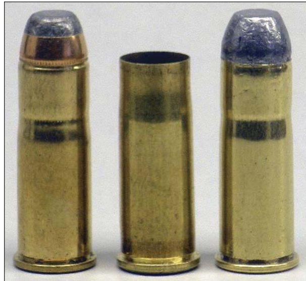
Winchester factory .44 WCF loads with jacketed (left) and lead (right) bullets are shown with a once-fired case that has been sized in a current full-length sizing die.
