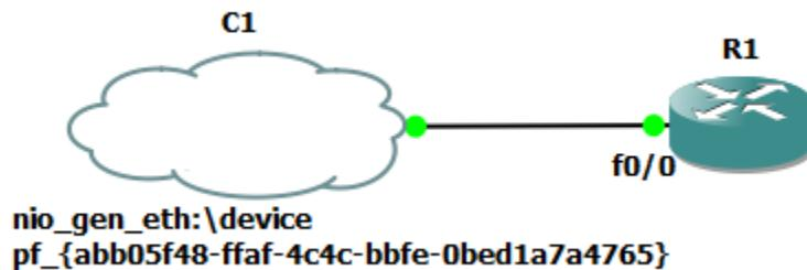
3. If your computer is connecting to the Internet using Wired Interface, configure interface f0/0 of R1 to obtain an IP address via DHCP. Otherwise, manually configure the IP address for R1's f0/0 interface. Assume f0/0 interface of R1 is allocated the IP address of 172.28.13.200
