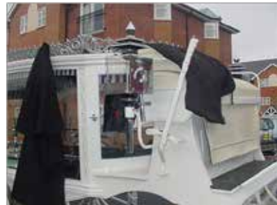
Fig. 1. An Oldsmobile horse carriage using lever type external brakes[1]
