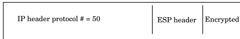
Figure 9-6 Packet with IPSec-Encrypted TCP Data
