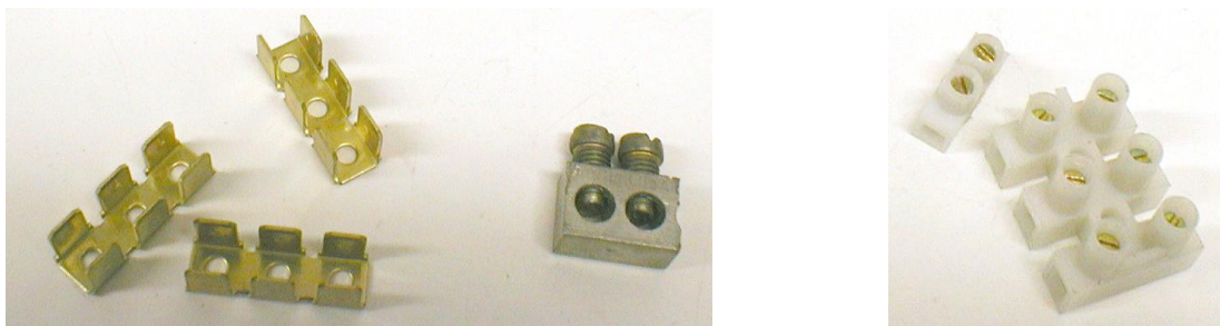
Figure 65: Various electrical connecting hardware: Left, spade type bus bars. These are used to connect all the primary windings in parallel. Middle, aluminum grounding bus bar cut into short lengths for connecting the high-amperage connections. Right, insulated terminal blocks for main power inputs.
