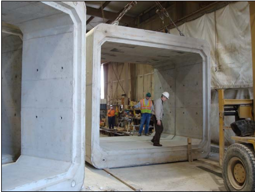
Figure 1: Concrete culvert inspection at the manufacturing facility.
