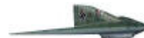
Horten XIIIb ( Year: 1944 Speed: 1200 Km/h; Altitude: 15.000 m; Motors: Heinkel He S 011 A-0 )
