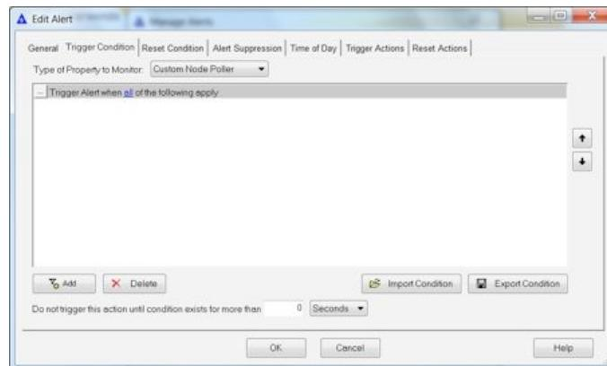
5. Click “Add” button in lower-right-hand corner, and select “Simple Condition”. Click on the first “\*” underneath “Trigger Alert when all of the following apply” and choose “Custom node pollers”, “PollerName”. Click on the second “\*” and enter “apStatus” to create the first trigger alert condition.
