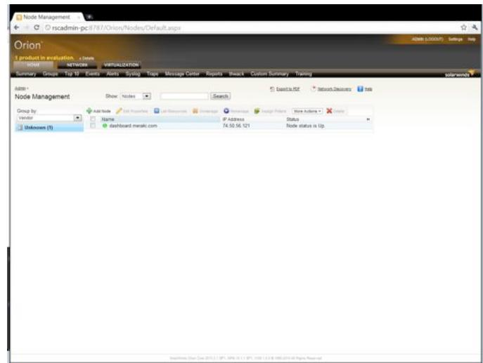
15. Click on “dashboard.meraki.com”. In the “Description” field under “Node Details”, you should see “Meraki Cloud Controller”. The Meraki Cloud Controller has now been added as a node to the Solarwinds Orion web console.
