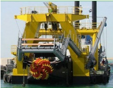
Cutter suction dredger
