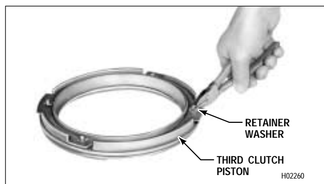
Figure 6–46. Removing Self-Locking Retainer Washers
