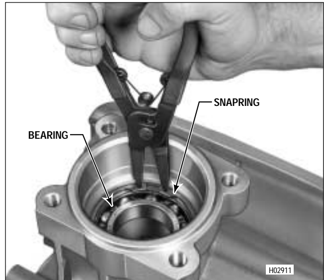
Figure 5-24. Removing Output Shaft Bearing Snapring
