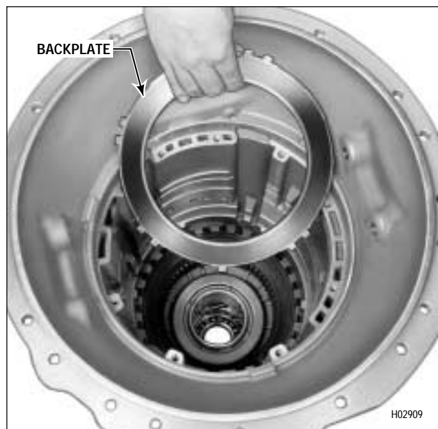
Figure 5-22. Removing Second Clutch Backplate
