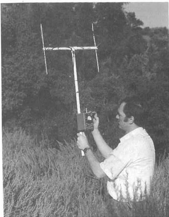
Fig. 12-9. The Sniff-Amp and Shrunk Quad can easily be held and operated with one hand.
