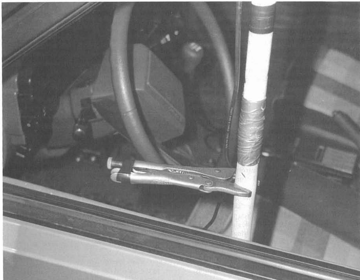
Fig. 7-17. One way to get a firm grip on the mast to turn it. Just be sure you clamp the pliers in the same direction each time.
