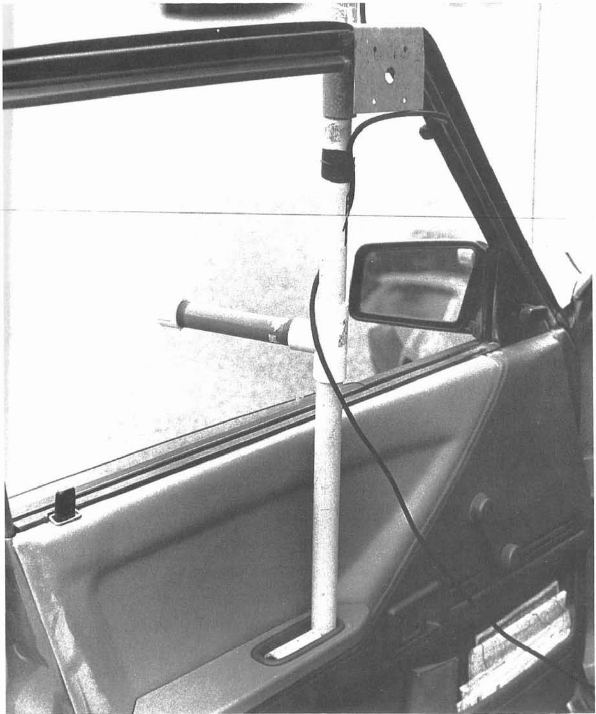
Fig. 7-16. A straight-forward handle and direction indicator combination. Note the top sheet metal bracket, held in place by closing the door on it. This is an outstanding example of a simple and cheap antenna mount that can be put together in a hour or two.
