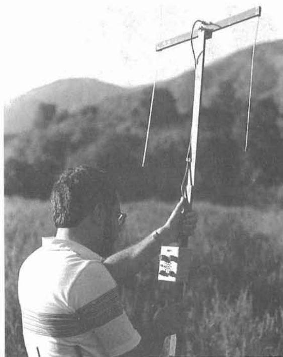
Fig. 8-4. Marc Wiz, WA6HBR, using the L-Per for sniffing.
