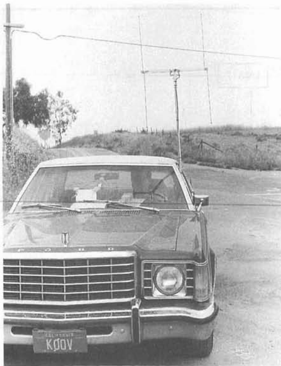
Fig. 7-28. Many states do not allow any overhang on the side of the vehicle. There is no overhang with this dual antenna DF.
