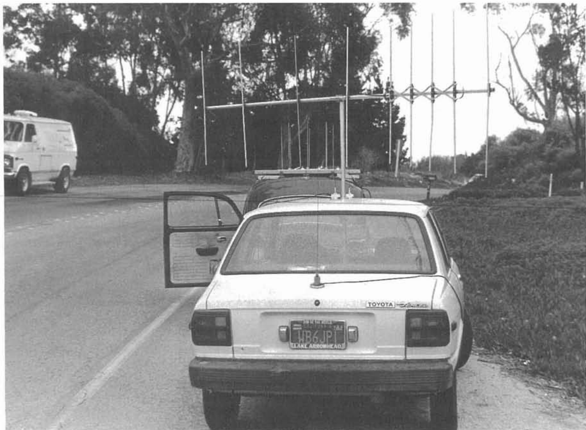
Fig. 4-4. WB6JPI hunts with a long KLM beam on a short car.
