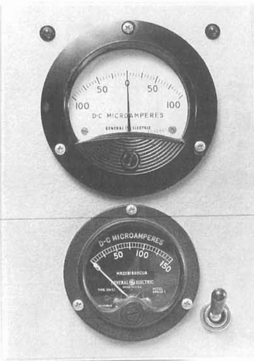
Fig. 8-11. The outside of a Happy Flyers DF. The top meter is the direction indicator and the bottom is the signal strength.
