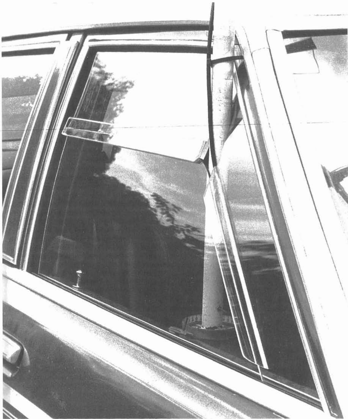
Fig. 7-15. When using a mount such as those shown in Fig. 7-5 or 7-6, a Plexiglas insert is an easy way to enclose the window. In certain installations it may need to be split and installed in two sections. Except for the hole and the split, the window is completely sealed. An insert of this type can easily be built in an afternoon.
