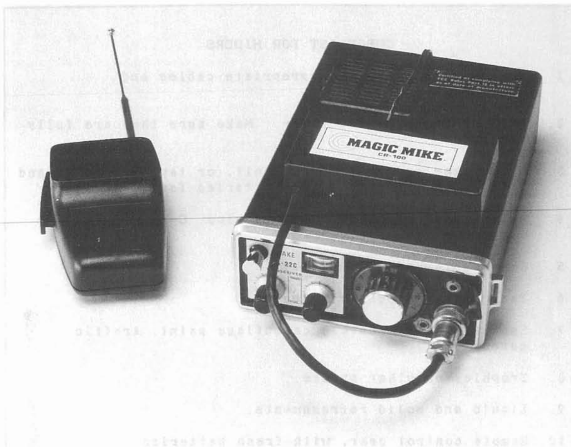
Fig. 14-21. A remote mike can be used to remotely talk through your T-hunt radio.
