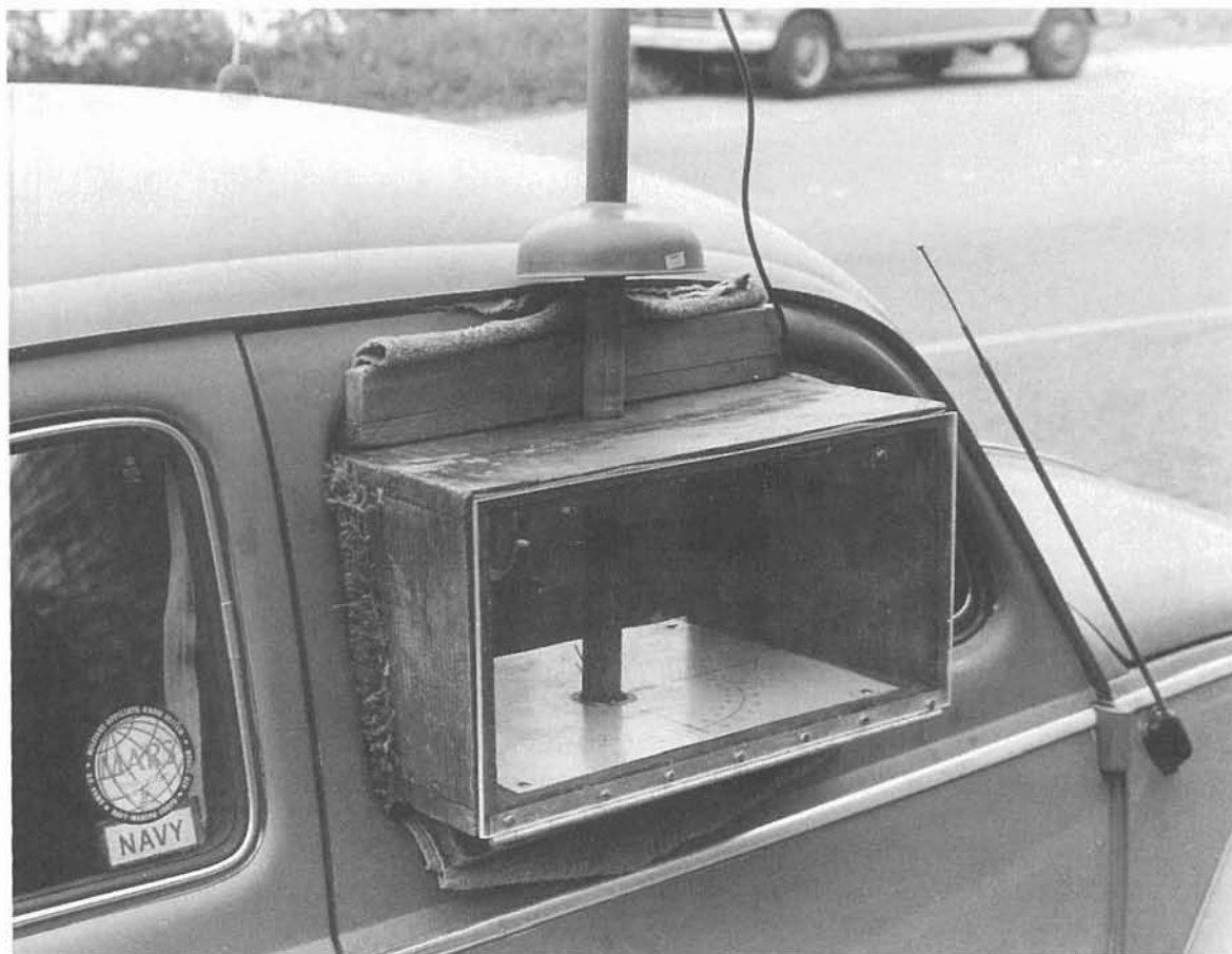
Fig. 7-14. A rather unusual window box, but it works. Note the "plumbers' helper" rain deflector and the large protractor around the base of the mast.
