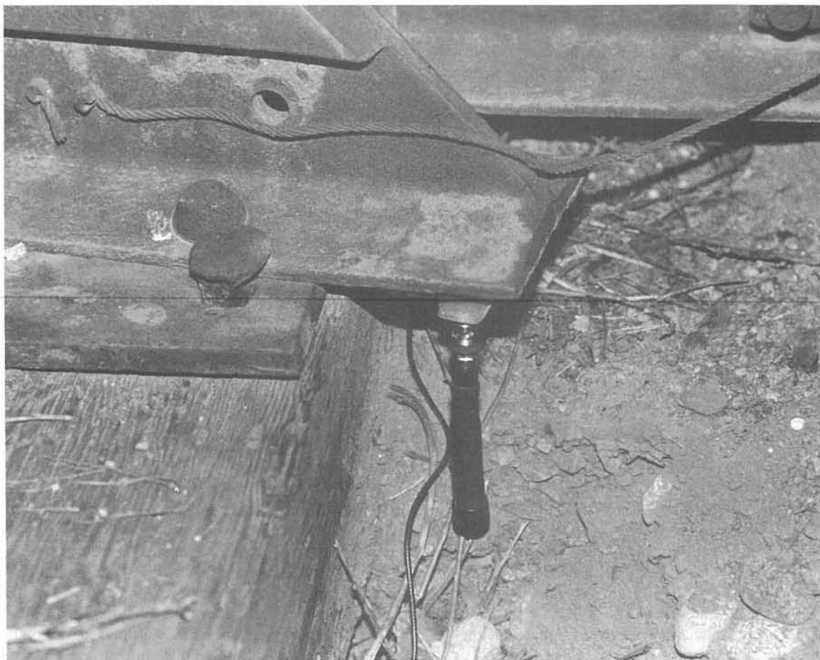
Fig. 9-16. The hidden T was hidden under the railroad bed; the antenna, a rubber duckie stuck to the bottom of the rail.
