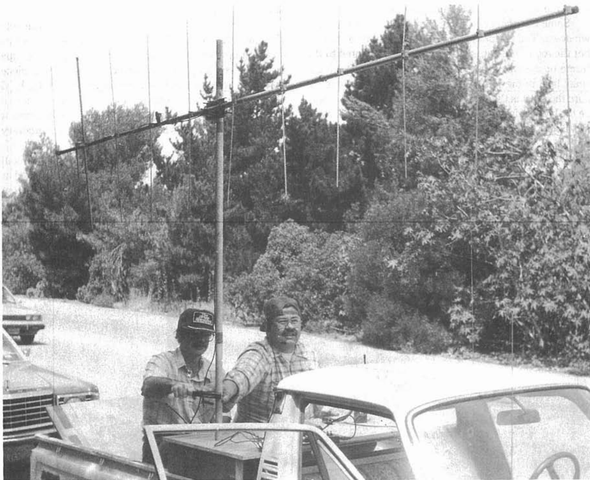
Fig. 7-3. John Schockley, WA6UVS, seats the navigator and beam turner in the rear of the pickup. The radio is mounted on the table, with attenuator and mast in easy reach. Note the headset to communicate with the driver.
