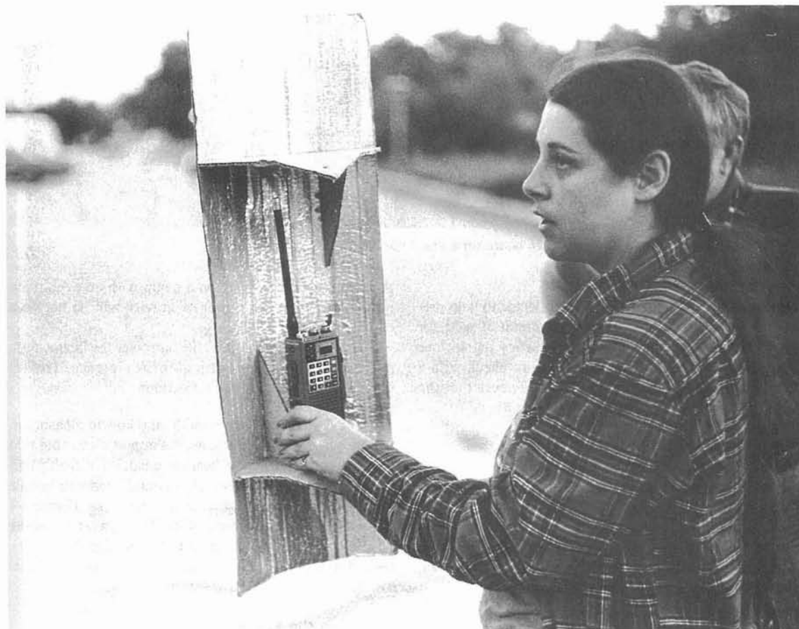
Fig. 4-3. Sally Lucas, KA6SYT, demonstrates a reflector for use with a 2 meter handheld.
