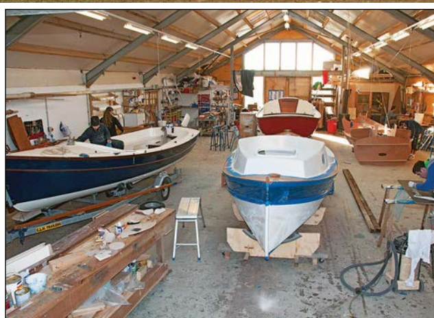
Above —The new Swallowboats workshop on the Teifi Estuary in Wales replaces the stone barn, to the right, where the business began. There's plenty of room now for a number of boats under construction, stationary power tools, and a CNC cutter. When the tide's up the boats can be launched and sailed right from the premises.
