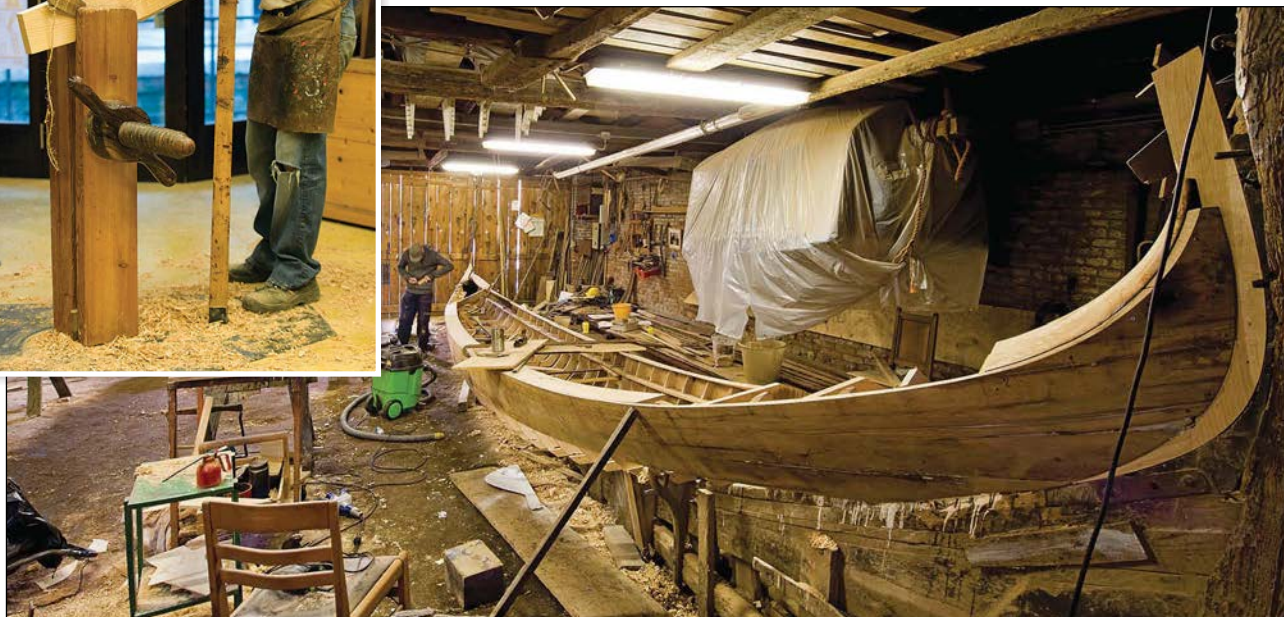
Above —At the Tramontin & Figli yard, Roberto Tramontin and his apprentice, Enrico, are building one of the two or so gondolas they produce each year. The yard was started in 1884 by Roberto's great, great grandfather Domenico Tramontin; it is credited with giving gondolas their asymmetrical form (see photo, page 73), which compensates for the fact that a gondola is always rowed with the oar on its starboard side.
