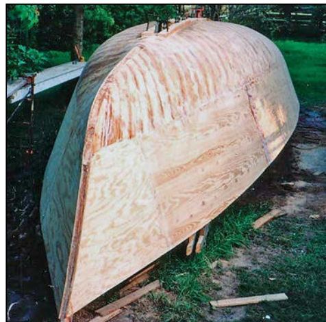
Left —The first Presto 36 in frame, being built by David West in Texas. Right —The same hull planked up, showing the transition from triple-laminated bottom to full-sheet plywood laminated topsides.
