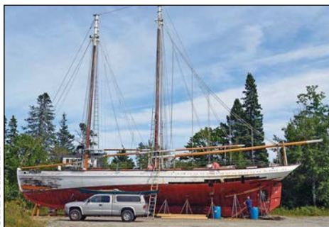
SYLVINA W. BEAL , a 1911 knockabout schooner now used for charters on the coast of Maine, was hauled out fully rigged for some planking and refastening.
