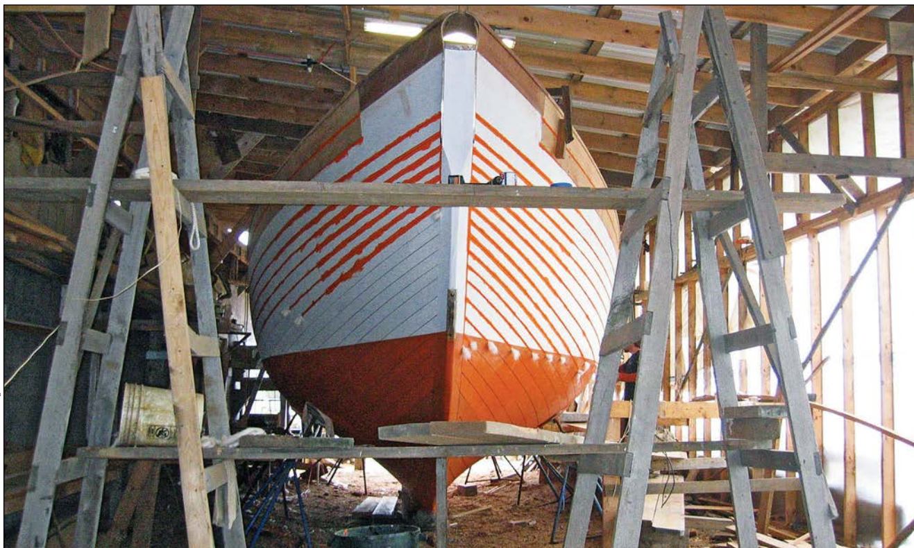
Here, caulking is progressing on the schooner's hull. The seams are then painted to keep the cotton from creeping, and to prevent it from absorbing the oils in the caulking compound that will be puttied into the seams.
