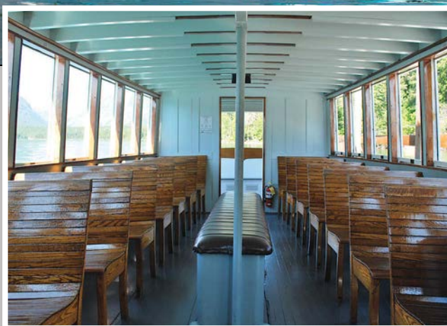
Above —The 56' DESMET was built in 1930 with red oak frames, which have since been reinforced with white oak sister frames. Planking is western red cedar. Left —The seats in all the boats are original, though these on DESMET have had to be reinforced owing to the increased weight of passengers.
