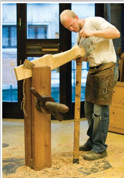
Left —Saverio Pastor's apprentice, Pietro Mengghini, working on a forcola. He is in the middle stages of creating its complex shape, removing wood with a large drawknife after the coarse form has been roughed out using a bandsaw. The workpiece is held in a large wooden vise fixed into the shop floor and supported with a strut at its extremity.
