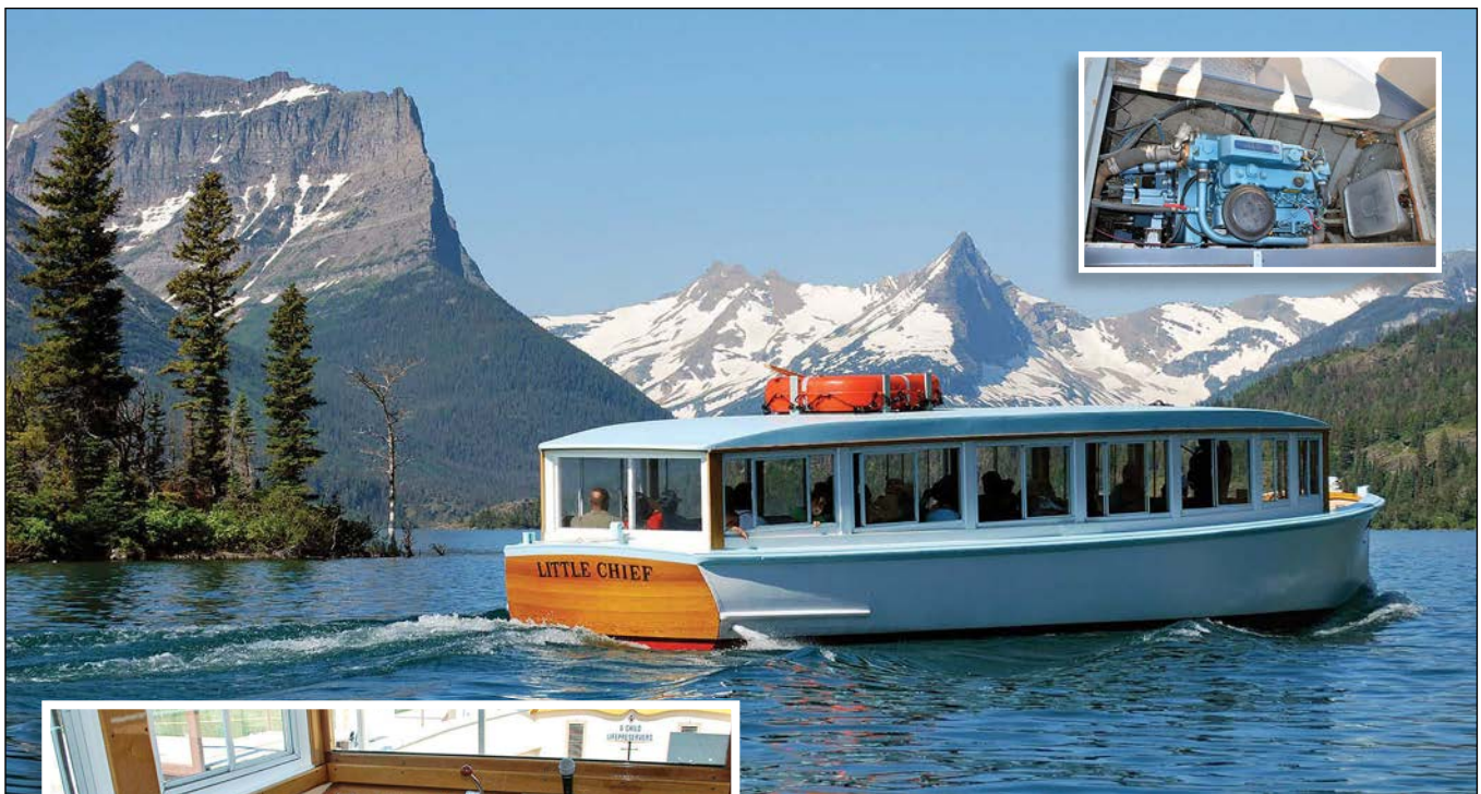
Above —LITTLE CHIEF, built in 1925 as a sistership to SINOPAH, makes daily runs on St. Mary Lake during the short tourist season. She's licensed for 49 passengers. Inset —As with all the launches, LITTLE CHIEF's engine is placed forward of the wheelhouse so as not to interfere with the cabin seating. Left —In the 1990s, the launch was restored and had her systems brought up to date so she could be placed back in service.
