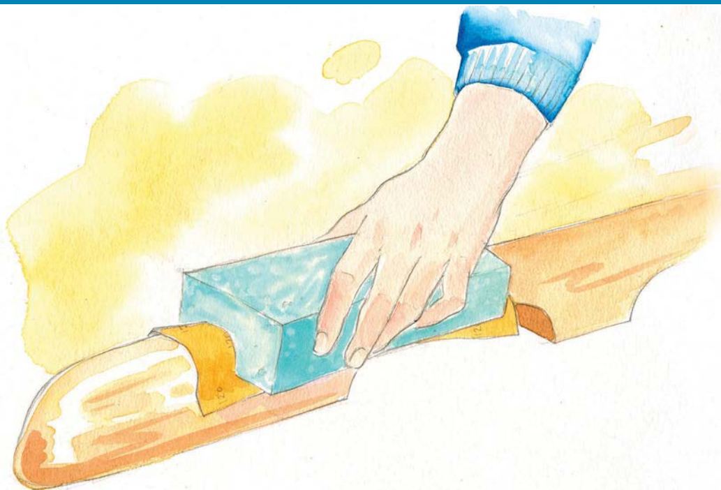
A block of foam insulation can be shaped to a contoured surface to create a custom sanding block.
