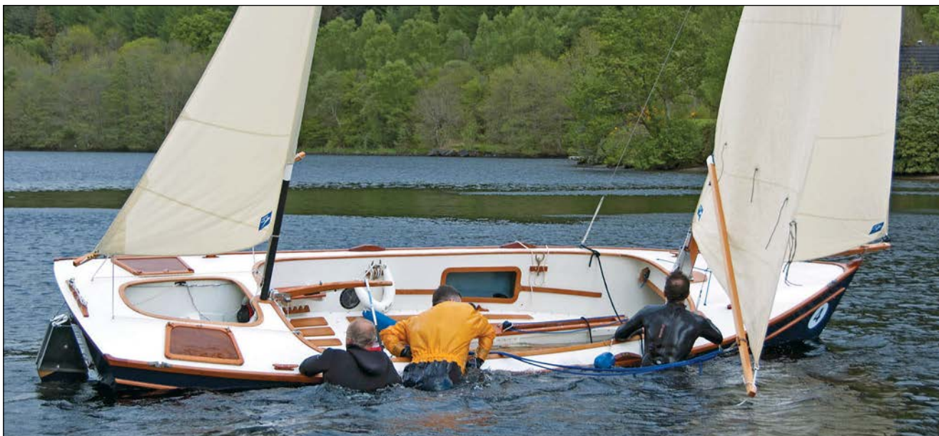
Crew climb back into the SeaRaider, CRAIC, after a capsize drill. With no water ballast in the tanks, the boat rights herself easily. Underway, with the tanks full of water, the boat is very stable under a press of sail.
