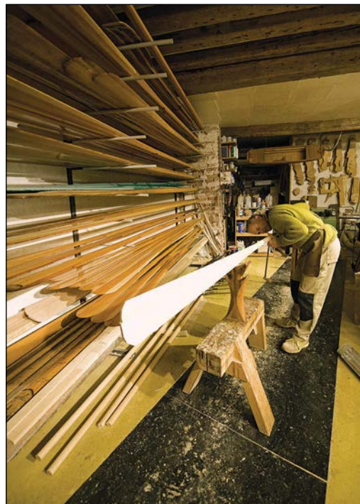
Above —Saverio Pastor shapes up a gondola oar in his workshop, which is situated along one of the canals in the Dorsoduro district. Here Savario checks the lines as the blade-end of the oar rests on a purpose-built support reminiscent of one of his forcola, set into a massive sawhorse. The oar is worked on with a variety of planes while its other end is being held in a floor-mounted vise just behind where he is standing.
