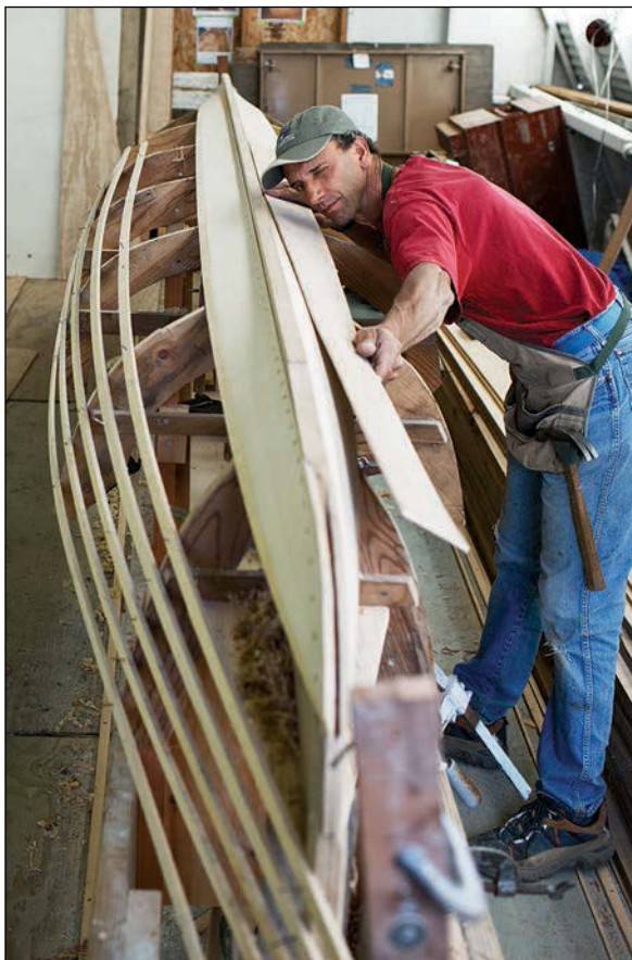
Above —By shaping patterns for each strake, Fisher-Smith made efficient use of his planking stock. Top right —For Fisher-Smith, lapstrake hull construction is all about carefully fitted planks; “they are key,” he says. Right —KOHLENBERG was built over the same molds used 23 years earlier for the construction of THOR.
