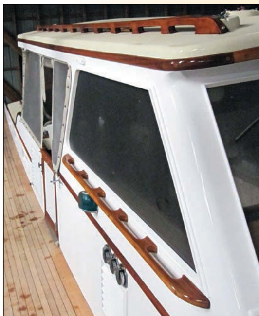
Above —On the C. Raymond Hunt-designed motoryacht STING RAY, handrails mounted on the pilothouse sides provide secure passage along narrow side decks.
