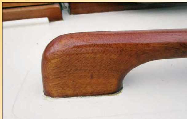
Right —End profiles should play off other joinery details found throughout a boat. Soft half-rounds are a typical detail on QUEST, a 42' yawl designed by John Alden and built by Paul Luke in 1959.
