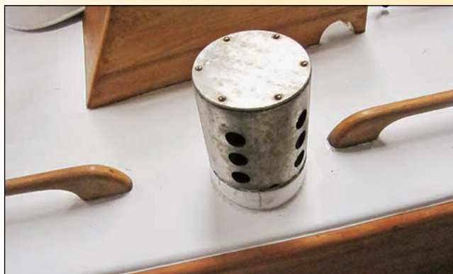
Left —It's best to simply stop and start a rail if it is interrupted by a piece of hardware, as is the case with this smoke head on the 46' Sparkman & Stephens yawl MADRIGAL. Don't be forced to move the rail inboard, where it will be less functional.
