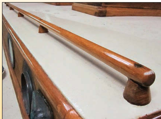
Above —CIRRUS, a Fishers Island 31 sloop built in 1931 by the Herreshoff Mfg. Co., carries a simple style of cabintop handrail first seen on Herreshoff yachts in 1912.
