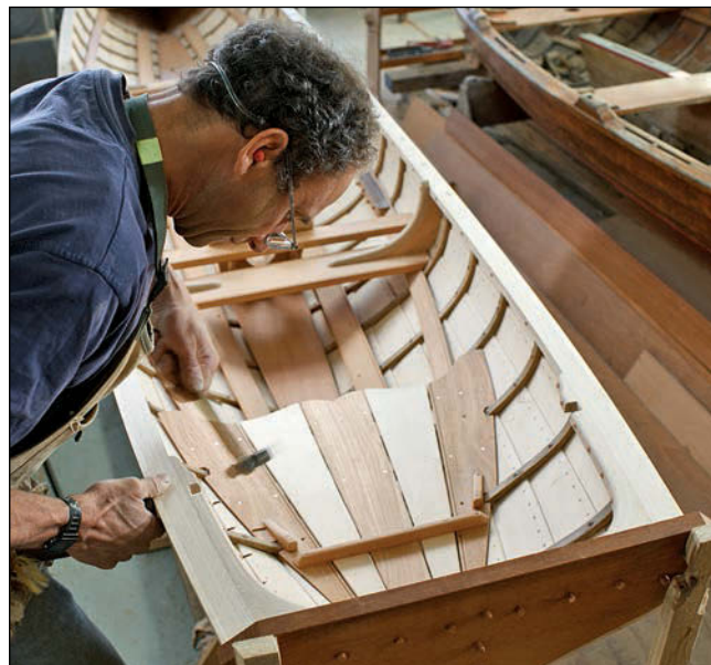
Top left —Fisher-Smith matched the construction details and scantlings of the original VIKING's hull but gave the new boat its own identity in such things as seat details. Left —Following the Bay Area rowing club tradition, the new boat's name is carved into her seat back. Above —KOHLENBERG's quarter knees are through-riveted into place.
