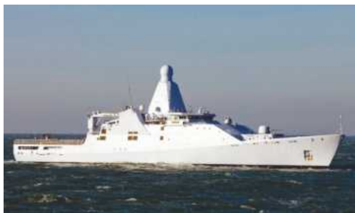
ABOVE Holland off the Dutch coast in 2012. An emphasis on good seakeeping in conditions found in the North Atlantic is reflected in the positioning of the bridge and accommodation areas towards the middle of the ship.
