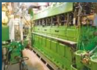
ABOVE Installed in 1983, Nordstjernen's MaK diesel drives her single screw.
