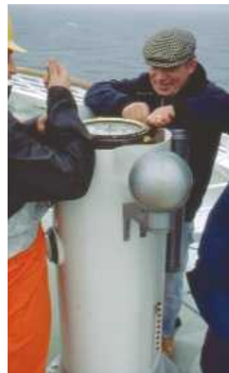
ABOVE Wärtsilä Shipyard's Trials Master and assistant fitting the magnetic compass.
