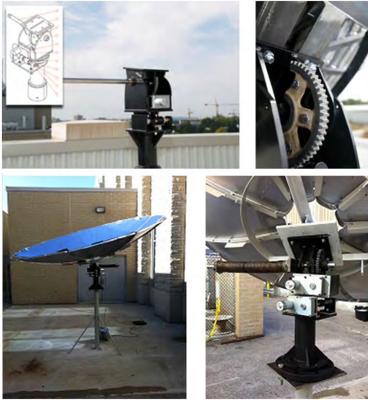
Figure 20.7 Solar tracker actuator technology with two main components, namely a dual-axis sun tracker means and a group bearing mechanism (WorlDiscoveries, 2014).
