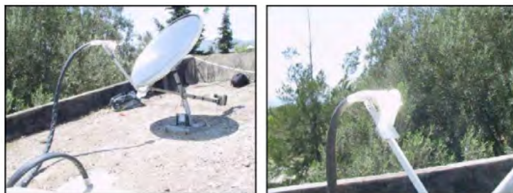
Figure 13.28 Transmission of concentrated sunlight in a fibre-optic bundle for solar lighting (Kandilli et al. , 2008).
