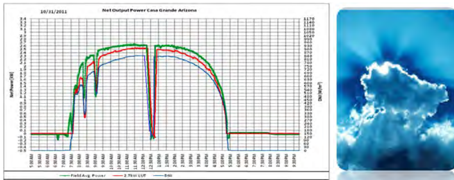
Figure 22.6 Hourly solar radiation and power generation curve for a solar receiver system operating in some overcloud conditions (Infinia, 2012b).
