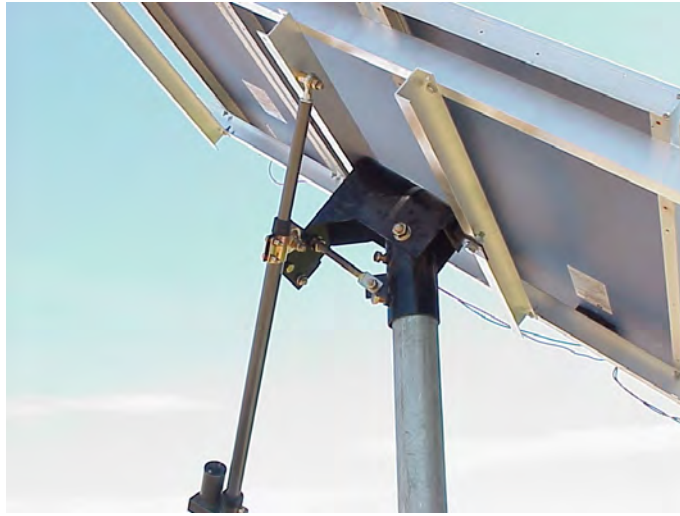
Figure 20.8 Solar tracker actuator technology working on the principle of Polar Tracking (Groene Energie, 2014).
