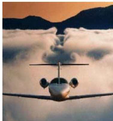
Figure 7. Downwash and wing vortices in the fog.
