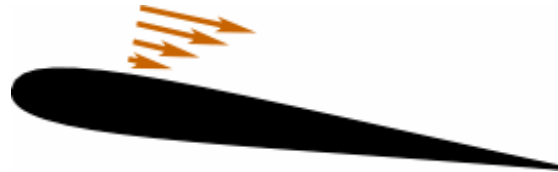
Figure 10. The variation of the speed of a fluid near an object
