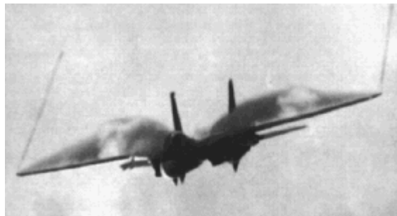
Fig 14. Condensation showing the distribution of lift along a wing.
