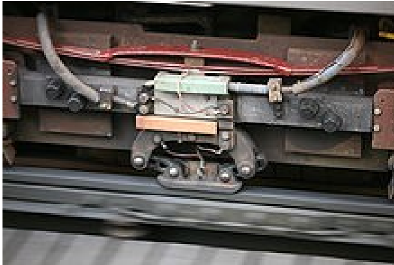
Chicago Transit Authority third rail contact shoe of Chicago 'L' car.
