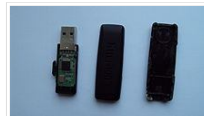
The internal mechanical and electronic parts of a Kingston 2GB flash drive
