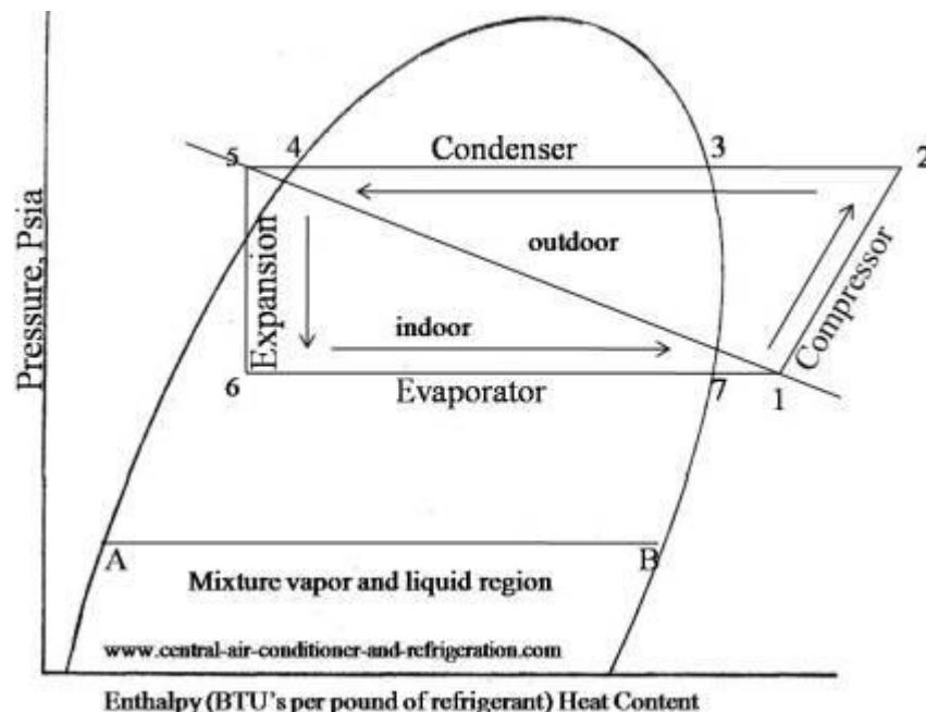
Point 2 on the pH diagram showed the hot vapor from the compressor is forced into the top of the condenser coils. The vapor refrigerant is being pushed at high speed and high temperature to the condenser units.
