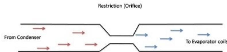
This is the basic principle behind any metering valves.
