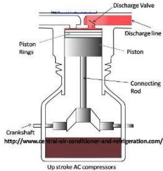
When the piston reaches the top of the cylinder, the discharge valve closes, and the suction valve opens as the piston starts down again drawing in cold refrigerant vapor to complete the cycle.
