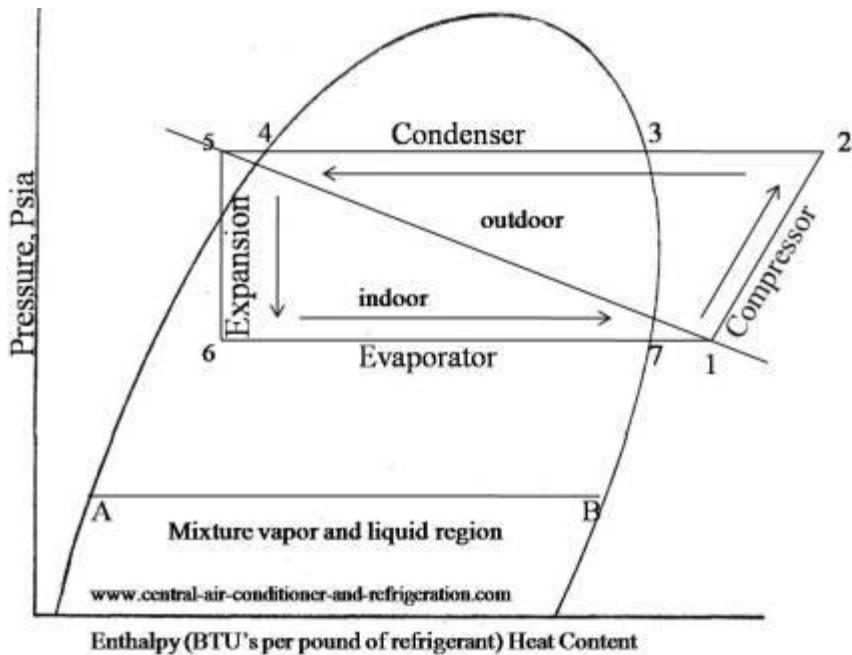
The process of the air conditioning compressors are showed between points 1 and 2 on the PH chart.
