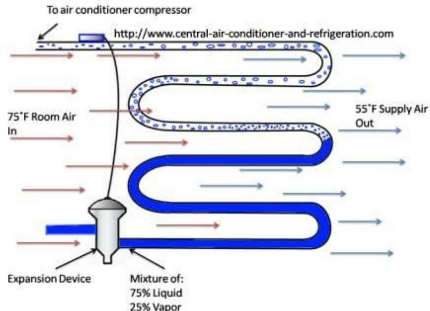
Air conditioning evaporator picture above tells us what happen to the evaporator coil.
