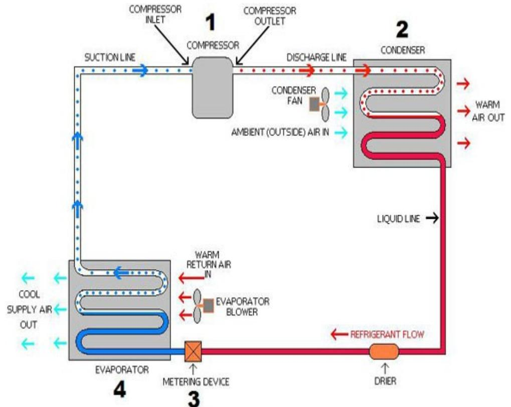
The component at #1 in this air conditioning circuit and cycle diagram is the compressor.
