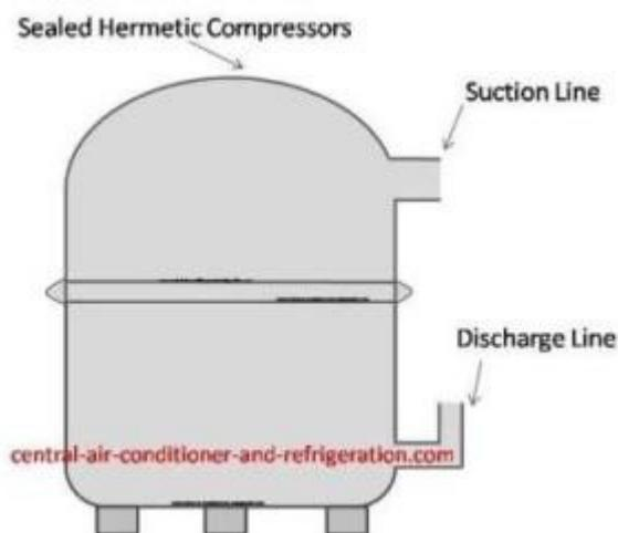
In a hermetic compressors there're two important tubes that welded with the hermetic shell. These two tubes are:
