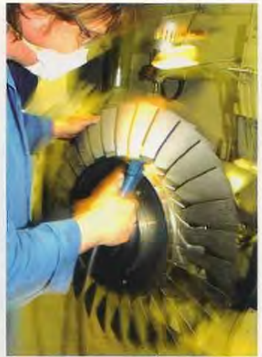
Fan blisk machined from solid on a 5-axis milling machine
