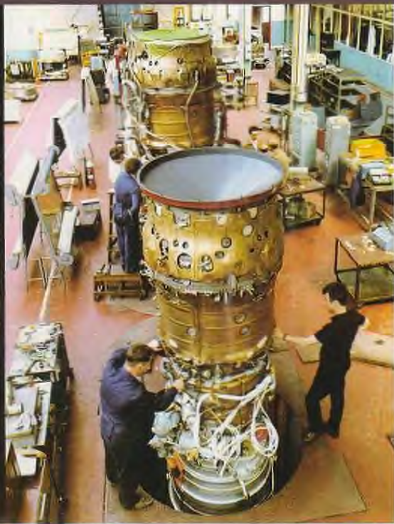
While most manufacturing techniques have seen dramatic changes over the last thirty years, the final assembly of an aero jet engine is still very much a highly skilled, hand-built operation.
