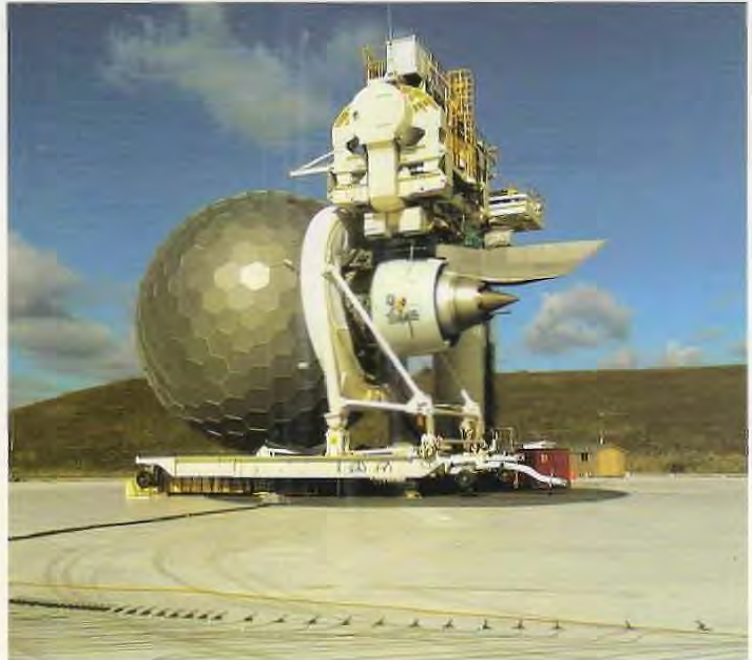
The acoustically transparent turbulence control screen used to remove atmospheric turbulence
