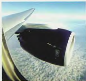
The Trent 800 short nacelle on the Boeing 777 gives separate jets for core and bypass flows
