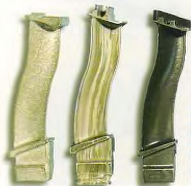
Three common turbine blade casting options balancing cost, yield, and performance: Equiax, directionally solidified, and single crystal alloys
