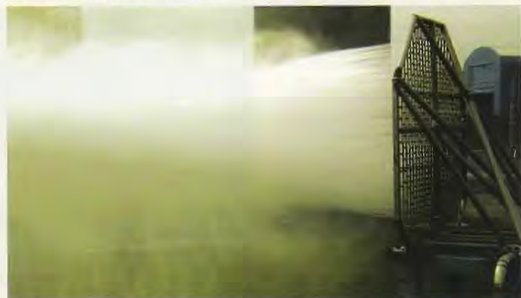
Rain ingestion testing with a full spray grid at sea level.
