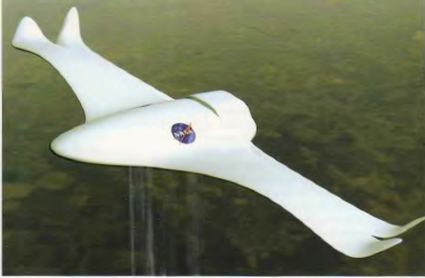
The 21st Century Aerospace Vehicle, aka the Morphing Airplane: NASA's concept for an aircraft using smart materials and technologies that could change its shape to suit different flight conditions*
