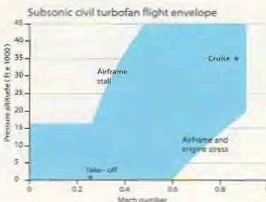
A typical operational envelope for a civil aero turbofan in terms of altitude and flight Mach number*
