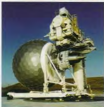
Use of the turbulence control screen on an outdoor rig with microphones arrayed around the engine.
