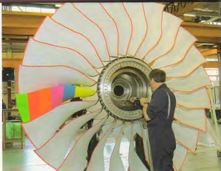
Preparation for a fan-blade-off test – the brightly coloured blade is released with an explosive charge.
