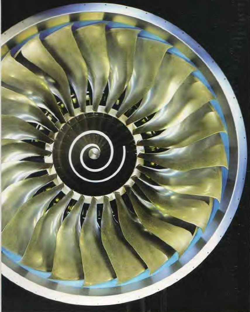
Wide-chord, swept fan blades on a high bypass turbofan
