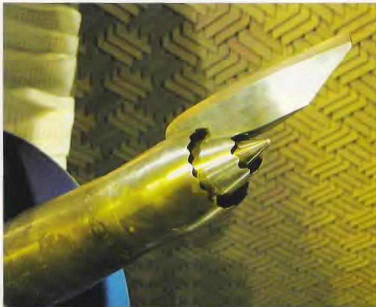
A model of a serrated nacelle and core in an anechoic chamber
