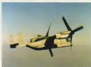
The V-22 Osprey takes off and lands like a helicopter, but can rotate its engine nacelles so that, in flight, it becomes a conventional high-speed, high-altitude turboprop aircraft
