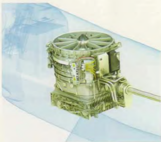
The two-stage, contra-rotating LiftFan® unit provides 18,000lbs of vertical thrust.
