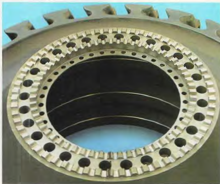
A Trent fan disc: the force locating a Trent fan blade is powerful enough to throw a car 30 metres into the air
