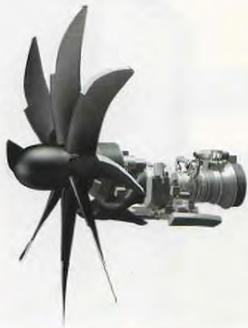
The TP400-D6 is the most powerful Western turboprop to date, with shaft horsepower in excess of 11,000shp.
