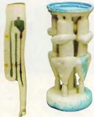
Right: A ceramic shell core that gives the complex internal cooling geometry to an HP turbine blade.
