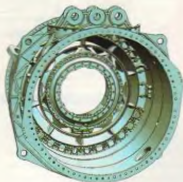
The intercase on a three-shaft engine, it locates the thrust bearings for all three rotors
