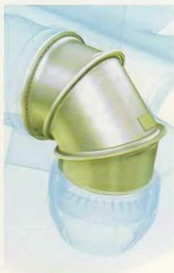
The 3 Bearing Swivel Module can provide 18,000lbs of vertical thrust in STOVL mode and rotates to give horizontal thrust for conventional flight.
