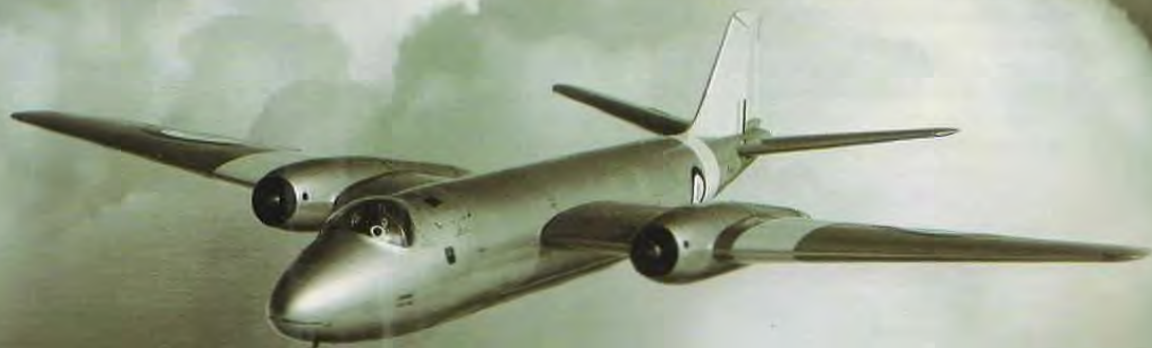
The English Electric Canberra, Britain's first jet bomber, made its first flight on 13 May 1949, powered by two Rolls-Royce Avon RA3 engines. It entered into service in 1951.
