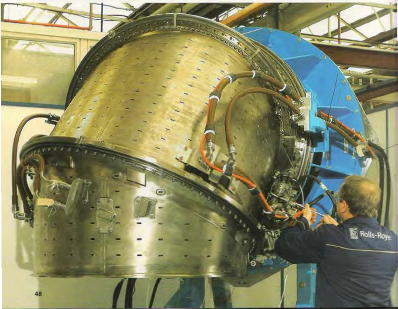
Preparing the 3 Bearing Swivel Module of the Joint Strike Fighter for testing
