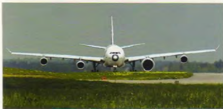
The A340 flying test bed with three of its original engines and one Trent 900 during its development programme for the A380
