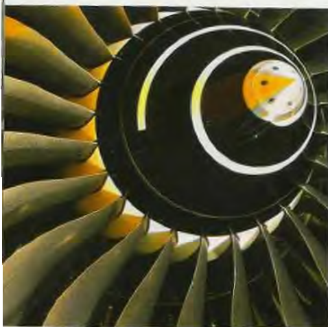
The swept fan forces the airflow into the more efficient centre of the blade passage
