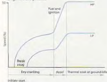
Engine start phases
