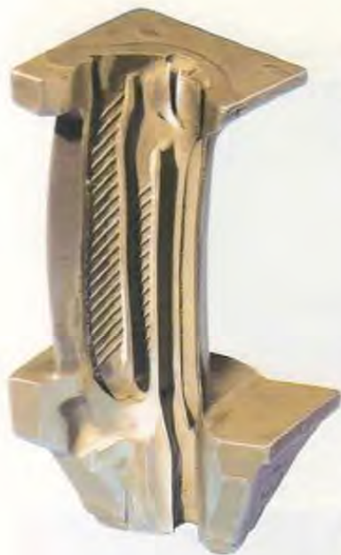
Left: A section through an HP turbine blade showing the complex cooling geometry after casting
