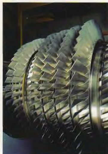
A Trent 800 IP compressor drum showing IP1 and IP6 stages without blades mounted.
