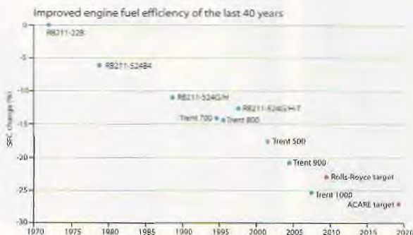
Levels of sfc have improved dramatically over the last 30 years, and will continue to improve in the future
