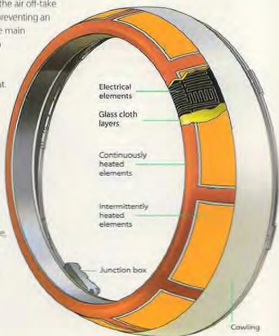
Electric de-icing components on the intake lip of a pitot nacelle
