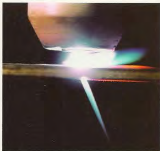
Welding with a plasma torch 13
