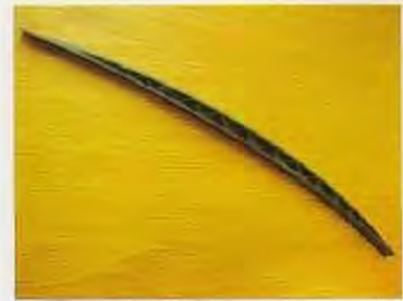
Section through a hollow fan blade
