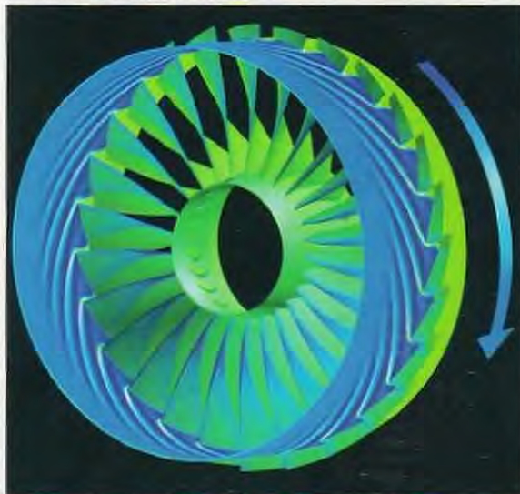
Slice through CFD solution showing pressure wave fronts travelling forwards from fan blades
