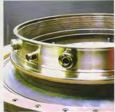
An example of additive manufacture by TIG weld deposition: an extended intercase, with bosses, prior to machining
