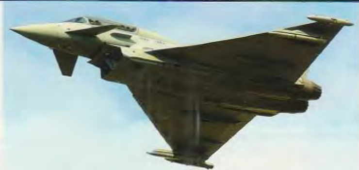
The under-fuselage-mounted supersonic intakes for the twin EJ200-engined Typhoon
