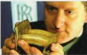
A development engineer examines a test turbine nozzle guide vane assembly
