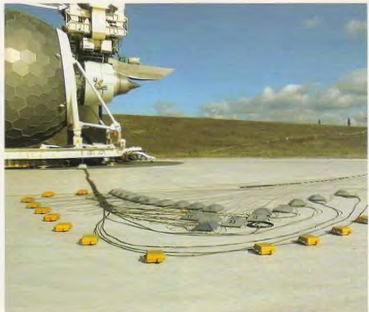
Some of the microphone instrumentation around an engine during a ground noise test
