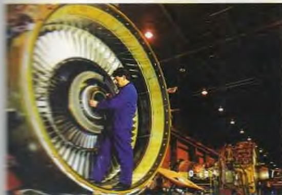
Final assembly starts with the fan case being connected to the core.
