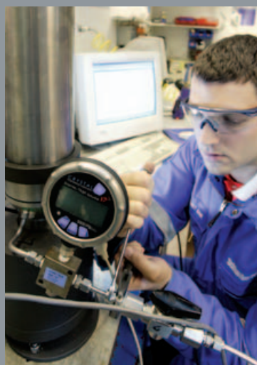
Pressure testing the Phoenix MultiSensor XT downhole gauge.
