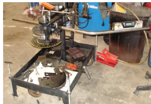
Figure 16: Hydraulic Bender used for fabrication
