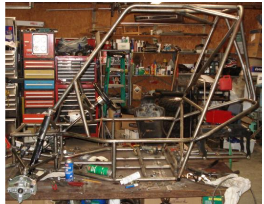
Figure 23: Frame with sub-assembly bolted up
