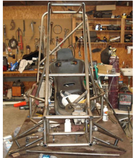
Figure 22: Aligning of front suspension arms
