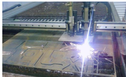
Figure 17: Plasma cutting of 3/16" plate
