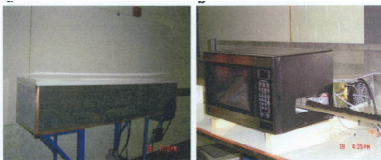
Fig. 5. (Left) Picture of the bench-scale microwave dewatering units with microwave shield in place. (Right) Close-up of the unit without the microwave shield showing the conveyor belt for feeding wet coal into the microwave oven (reproduced from the paper by Seehra et al., Fuel 2007).
