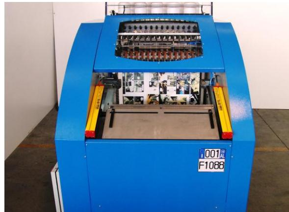
The manual book sewing machine is operated by front loading of signatures. The machine is equipped with an automatic cutting system using fixed knives with blind stitch by means of vacuum between the book blocks. The operator friendly system facilitates the separation of the book blocks on the exit delivery table.
