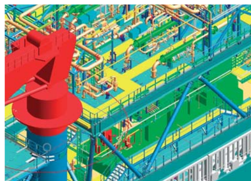
Close-up details of two of the topsides modules modelled with AVEVA PDMS. Image courtesy of Aibel
