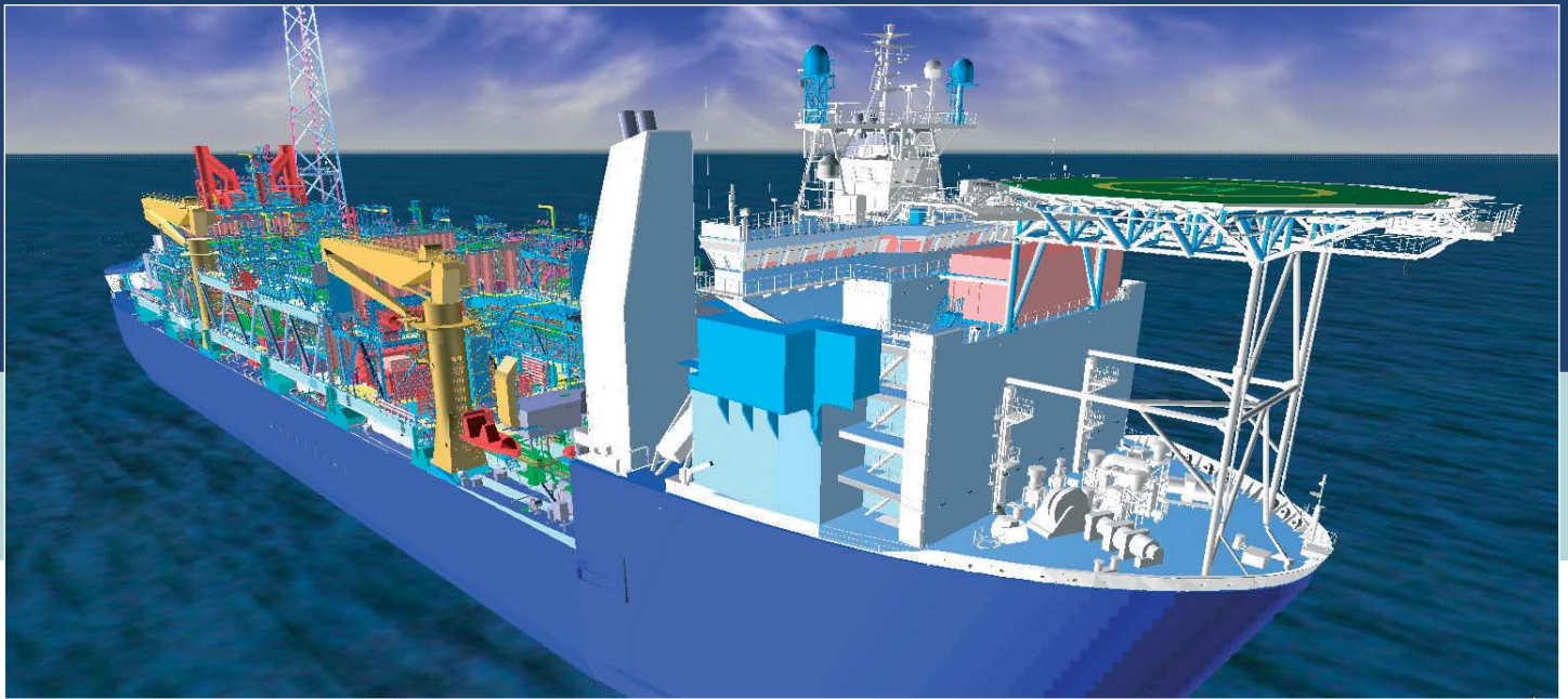
The Alvheim FPSO – the original deck structure was laser scanned to aid the integration with the topsides modelled with AVEVA PDMS. Image courtesy of Aibel
