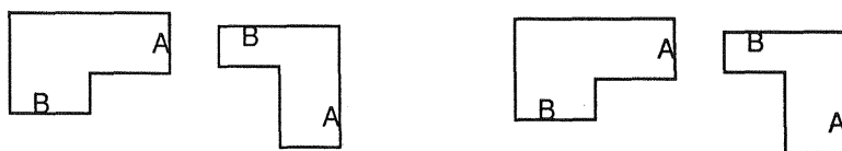
Fig. 24 Schematic of an example of molecular arrangement possibilities in a crystalline solid. If groups A and B can interact, then the situation in the upper arrangement is less prone to reaction, since A and B are at a greater distance.
